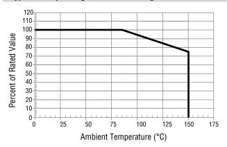
This graph shows the typical device surge current derating versus ambient temperature when subjected to the 8/20  $\mu$ s current waveform per the IEC 61000-4-5 specification. This device is not intended for continuous operation at temperatures above 125 °C.
